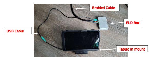
The back of the ELD has 4 USB ports around the outside. Your devices (tablet/camera) should already be plugged in to USB ports. Any of these can be used for charging, and may have rubber stoppers in them that must be removed before plugging a device in. The braided cable light in the middle of the ELD box should be green if it is powered on and properly connected to Wi-Fi.
